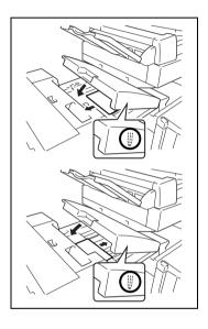
4 If finisher F-8430 is installed, open right-side door FN7.
